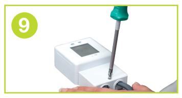
Refit the cover onto the front of the timer unit.
