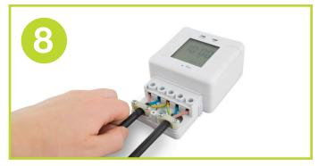
Test that the wires are fixed in properly by pulling on the cable. If a wire comes loose, repeat from step 6.
