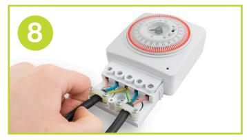
Test that the wires are fixed in properly by pulling on the cable. If a wire comes loose, repeat from step 6.
