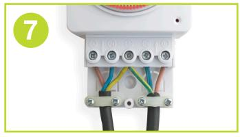
Fully tighten the terminal screws and make sure that no bare copper is exposed outside of the terminal.
