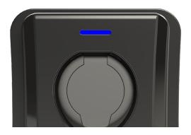
In less than 2 minutes, the indicator should turn from Yellow to Blue to confirm network connection.
