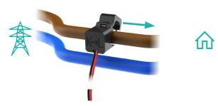
Open the CT Clamp and fit around the incoming Live power cable, this is typically marked brown for most installations.
